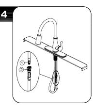
Align male fitting (1) and tabs (2) on quick connector. Push quick connector housing firmly upward and snap onto receiving male fitting. Pull down moderately to ensure connection has been made.
