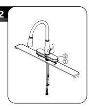
Optional Deck Plate Installation: Before installation, remove the flange. Align the hole in the gasket (1) and deck plate (2) with the mounting hole in the sink. Place the faucet assembly through the deck plate (2) and mounting hole in the sink until the faucet assembly sets on top of deck plate (2). NOTE: If the sink is uneven, use silicone under the gasket (1).
