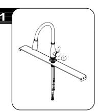
Optional Flange Installation: Before installation, ensure that the flange (1) is placed on the bottom of the new faucet assembly. Insert the faucet body through the hole in the sink.
