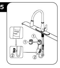
Install the weight clip (2) at the point of the hose marking "Weight here". Insert the weight (1) onto the clip (2) by sliding it down onto the clip (2).
